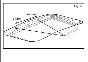
From the center mark measure 142mm to each side and mark a line on the flange using a felt tip pen.
