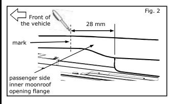
5) Measure 28mm forward from edge shown on passenger side inner moonroof opening flange and mark location on flange using felt tip pen. Repeat for driver side.
