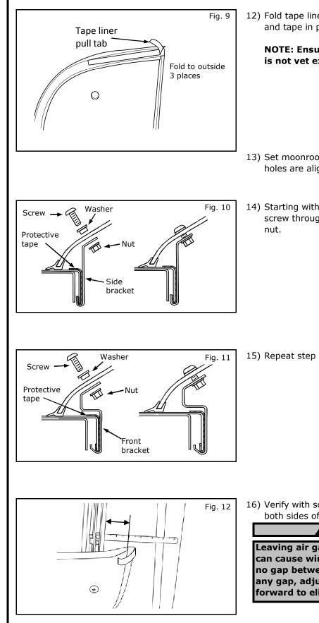
12) Fold tape liner pull tabs to outside of deflector and tape in place.
